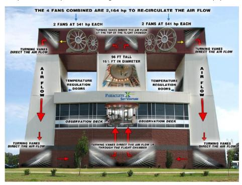
The picture below provides an integrated view of the structure and equipment.
